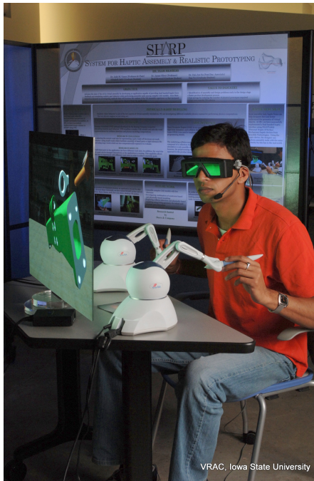
Figure 6: Dual-Handed Haptic Configuration for SHARP
