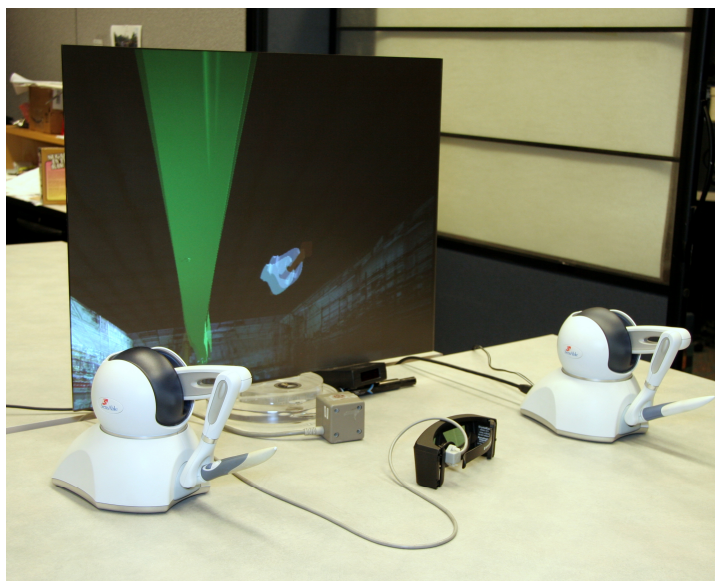
Figure 28: Desktop VR Setup with 2 Phantom Omnis
